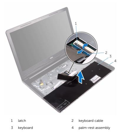
6 Lift the keyboard, along with the cable, off the palm-rest assembly.
