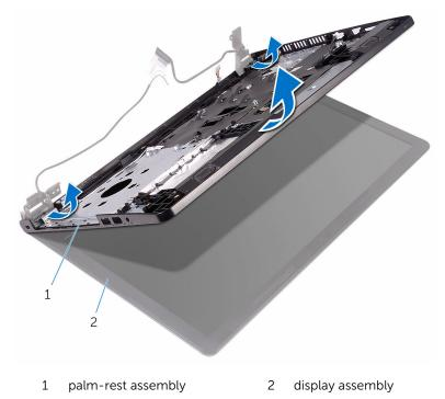
6 Place the display assembly on a clean, flat surface.
